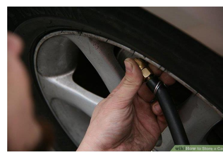
**Inflate the tires to proper pressure.** If you are storing for the winter in a cold climate, check the manual for proper pressures.Over inflation while in storage may help to prevent flat spots. After storage expect some thumping tires until they are driven 10 miles (16 km) or so.
