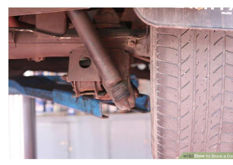
If the car will be stored for extended periods of time, it is advisable to jack it up on axle stands to avoid flat spots in the tires. "Extended" in this case depends on the type of tires; bias-ply tires need to be jacked up sooner than radials, and high-profile sooner than low-profile. A "classic" car with fat bias-ply tires should be jacked up if stored for more than a month, a modern sports car with low-profile radials should be fine for a winter.
