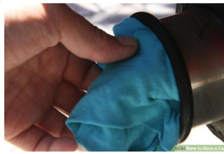
**Open a window slightly if stored indoors, but not enough to allow small animals inside.** Put the top up if it's a convertible. Stuff a rag into the air intake and exhaust to prevent animals from nesting, covering this with a metal screen (1/4 inch square screen is useful here). Some suggest using strong-smelling chemicals like soap or mothballs to keep animals away, but these can leave a smell in the car.
