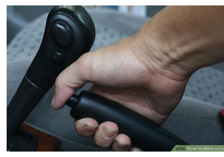
**Release the handbrake.** If the brake is left on, the brake pads can stick to the rotors. Place chocks under the tires to prevent movement, which is even more effective than the brake, anyway.
